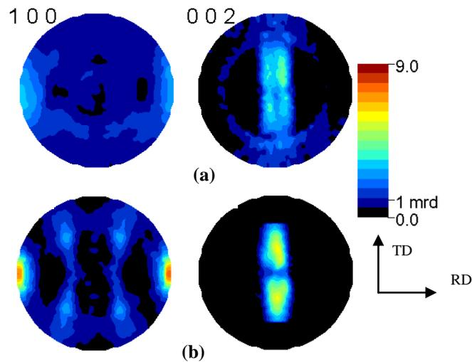
Figure 1: Initial (a) and final (b)  $\{0002\}$  and  $\{10\bar{1}0\}$  PF.
