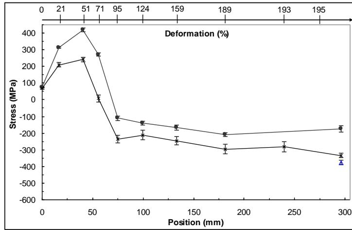
**Figure 2:** experimental longitudinal stress  $\sigma_{11}^{\text{exp}}(\text{hkil})$  calculated with the relation (6) ( $\langle \varepsilon^{\text{Ipi}}(\phi, \psi, \text{hkil}) \rangle_{V_d} = 0$ ) and obtained with different crystallographic planes. (a):  $\blacksquare$ - $\{10\bar{1}4\}$ ,  $\square$ - $\{20\bar{2}2\}$ ,  $\bullet$ - $\{0004\}$  (with Cr radiation). (b):  $\bullet$ - $\{20\bar{2}5\}$ ,  $\Delta$ - $\{30\bar{3}2\}$ ,  $\times$ - $\{21\bar{3}3\}$  (with Cu radiation).
