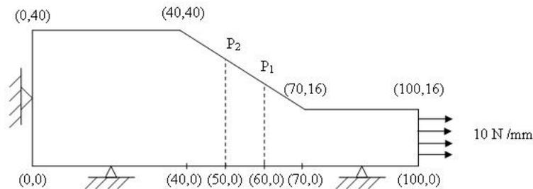
**Figure 3.** Example of a plate.
