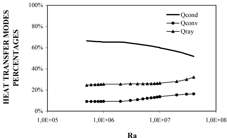
**Figure 8:** Contribution of different heat transfer modes to the overall heat flow through the honeycomb wall.
