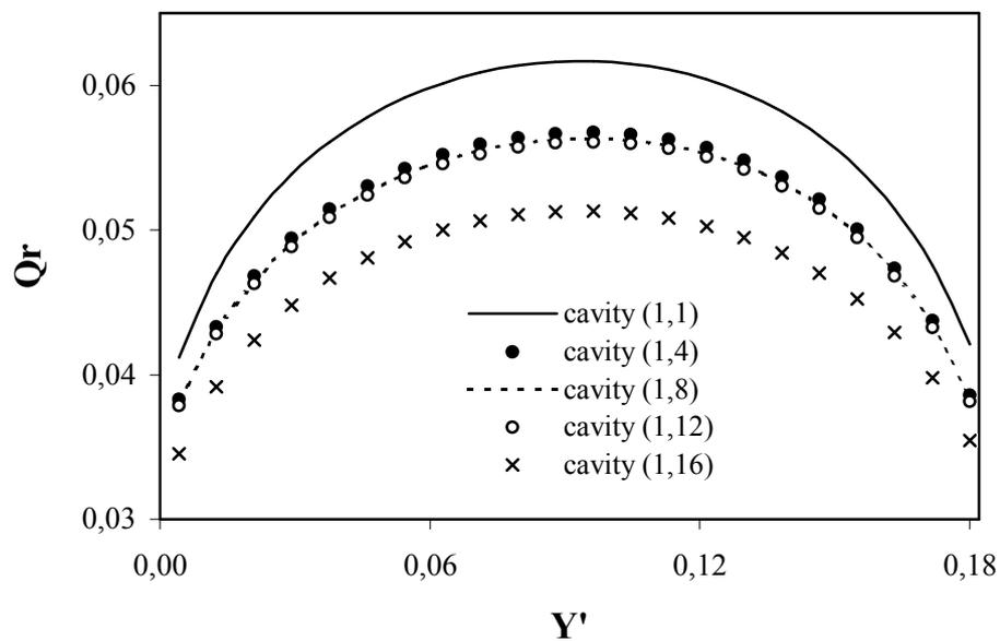
**Figure 6:** Variation of the dimensionless radiative heat flux along the left vertical side of the first vertical cells range.
