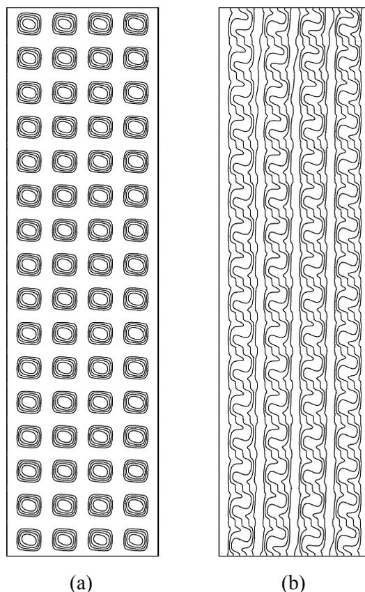
**Figure 2:** Streamlines (a) and isotherms (b) obtained for  $N_x=4$ ,  $N_y=16$ ,  $Ra=2.53 \cdot 10^7$ ,  $G=1.14$  and  $Nr=3.27$ .
