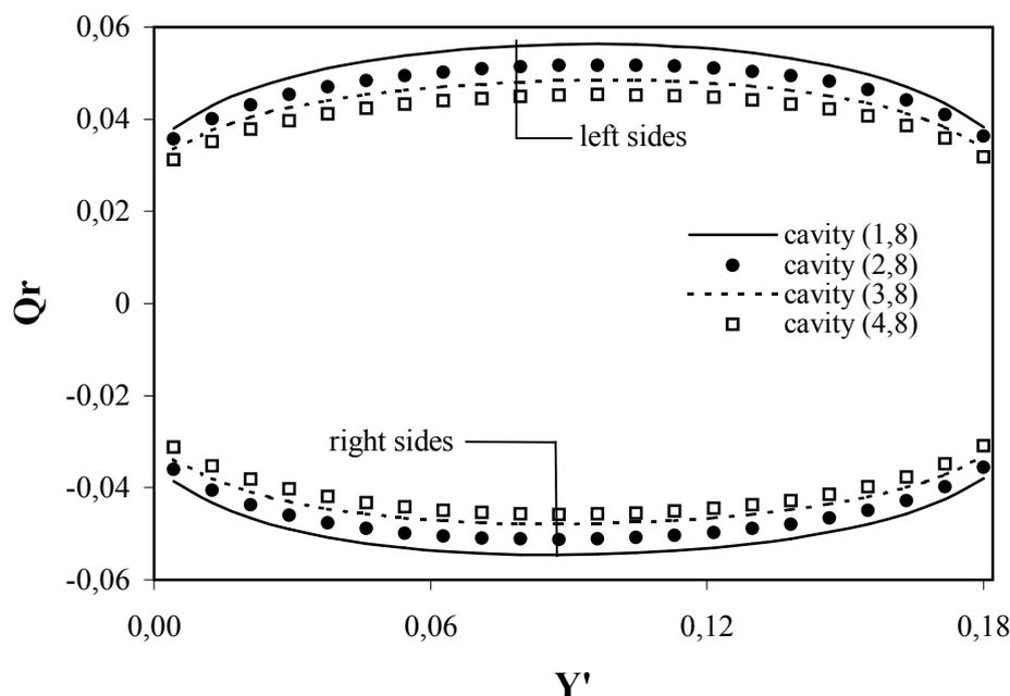
Figure 4: Variation of the dimensionless radiative heat flux along the vertical surfaces.
