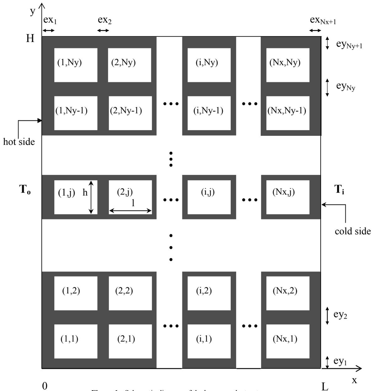
Figure 1: Schematic diagram of the honeycomb structure.
