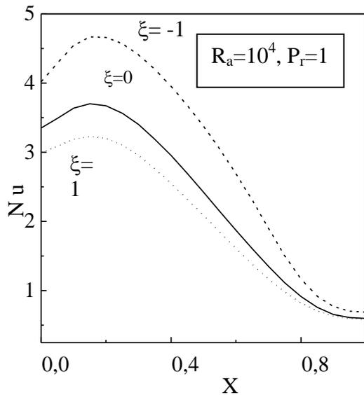
Figure 14: Nusselt number variation along the heated wall for various  $\xi$
