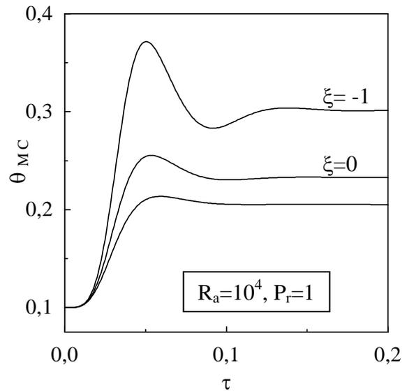
**Figure 11:** Transient temperature at the midplane of the cavity near the cooled wall for various  $\xi$
