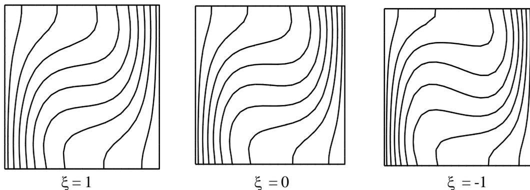
**Figure 5 :** Isotherms for  $P_r = 1$ ,  $R_a = 10^4$  and for three relative values of  $\xi$
