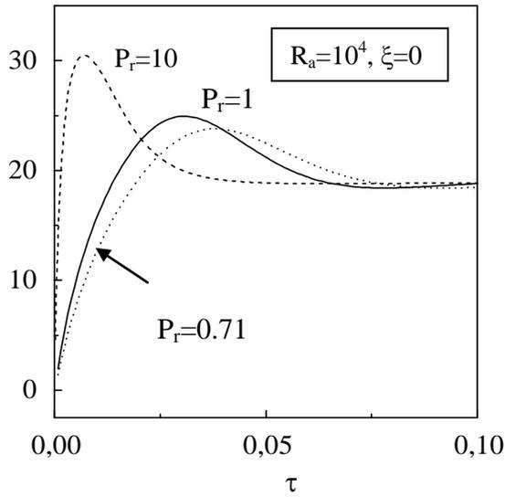
**Figure 8 :** Transient velocity at the midplane of the cavity near the heated wall
