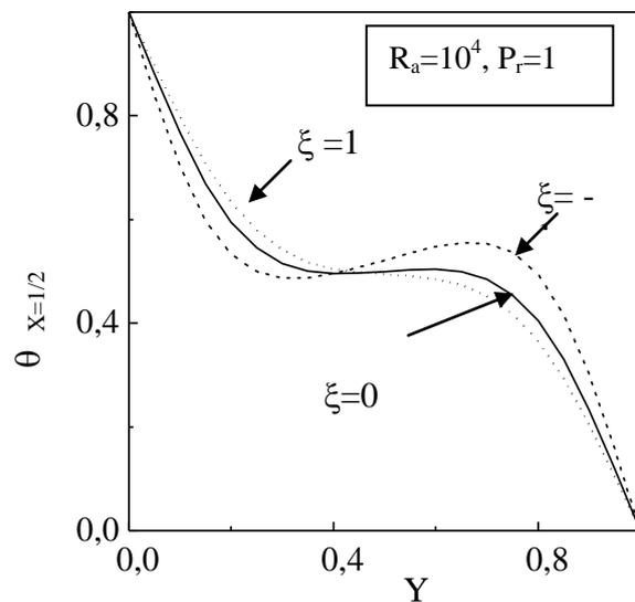
**Figure 7:** Temperature profile along Y for various  $\xi$
