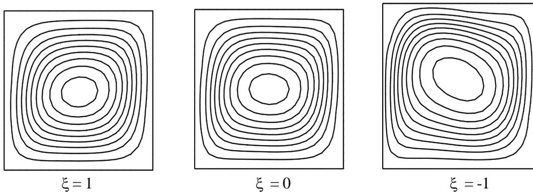
**Figure 4 :** Streamlines for  $P_r = 1$ ,  $R_a = 10^4$  and for three relative values of  $\xi$
