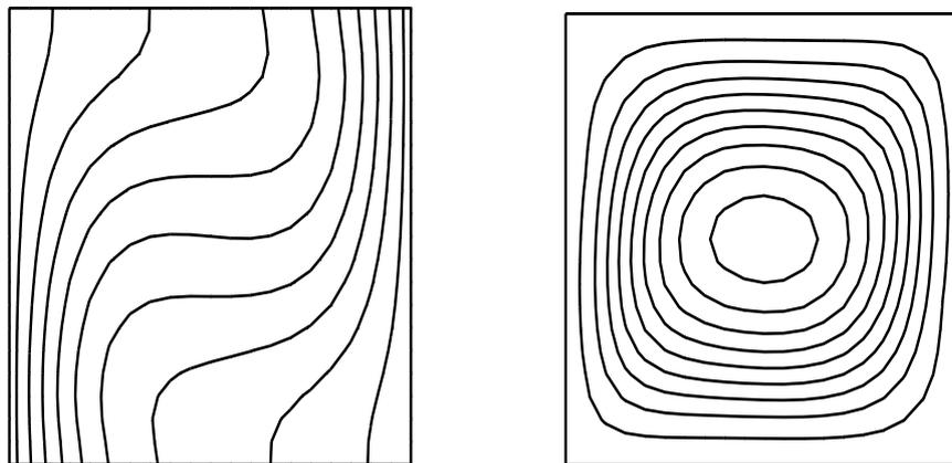
**Figure 2:** Streamlines for  $P_r=1$ ,  $R_a=10^4$  and  $\xi=0$  **Figure 3:** Isotherms for  $P_r=1$ ,  $R_a=10^4$  and  $\xi=0$
