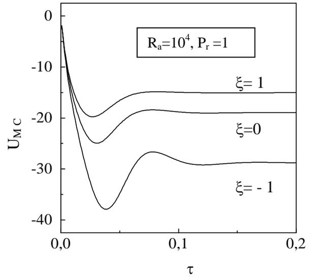
**Figure 9:** Transient velocity at the midplane of the cavity near the cooled wall for various  $\xi$
