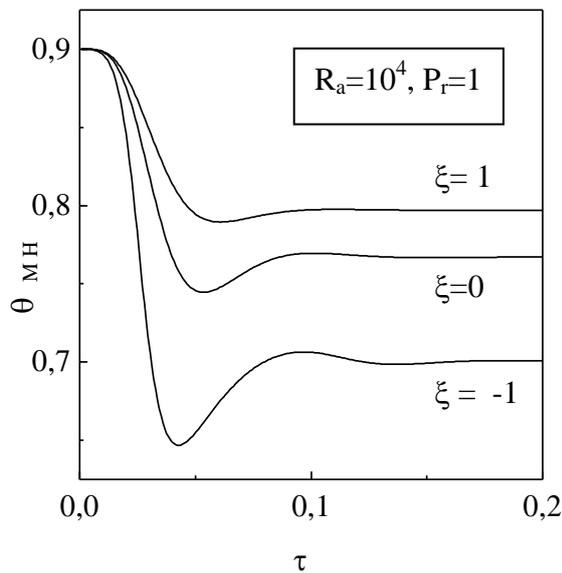
Figure 12: Transient temperature at the midplane of the cavity near the heated wall for various  $\xi$
