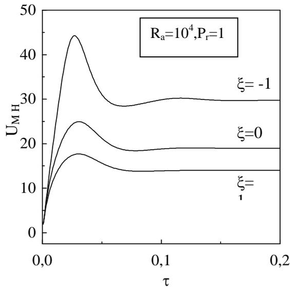
**Figure 10:** Transient velocity at the midplane of the cavity near the heated wall for various  $\xi$
