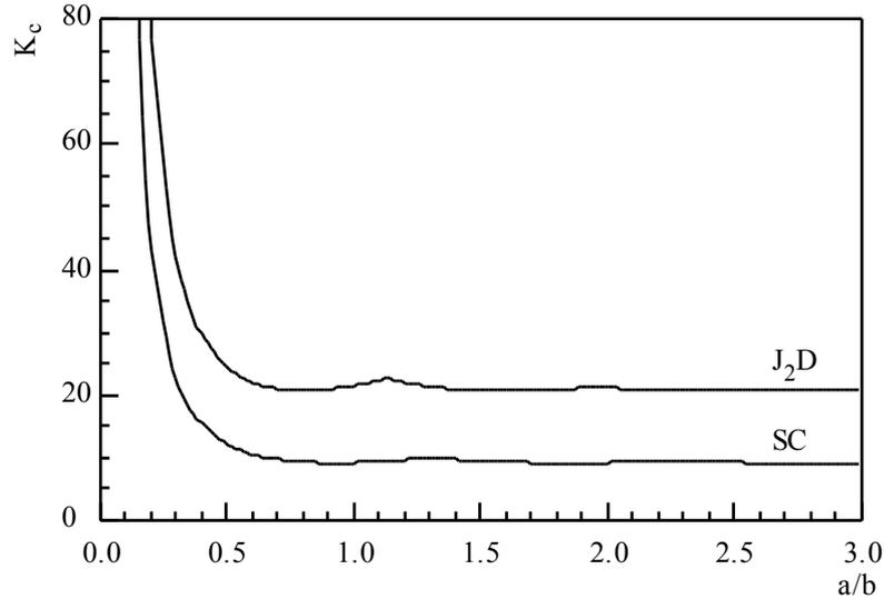
**Figure 8-b:**  $K_c$  versus aspect ratio  $a/b$  for the deformation theory and for the self-consistent model when the applied plastic strain is 1%.
