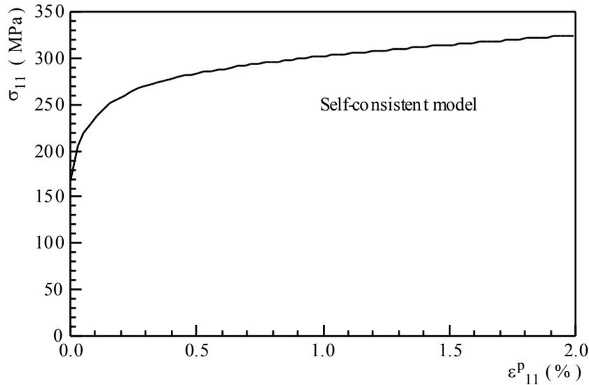
**Figure 2:** Stress strain curve obtained by the self-consistent model.
