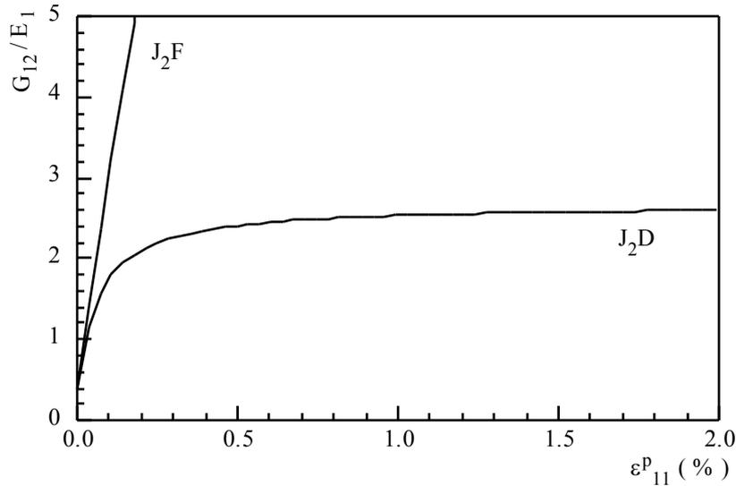
Figure 1-5: Evolution of the ratio  $\frac{G_{12}}{E_1}$  for the models  $J_2F$  et  $J_2D$ .
