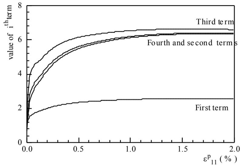
**Figure 11-b:** The four terms of  $K_c$  versus plastic strain according to  $J_2D$  theory and with an aspect ratio  $a/b = 1$ .
