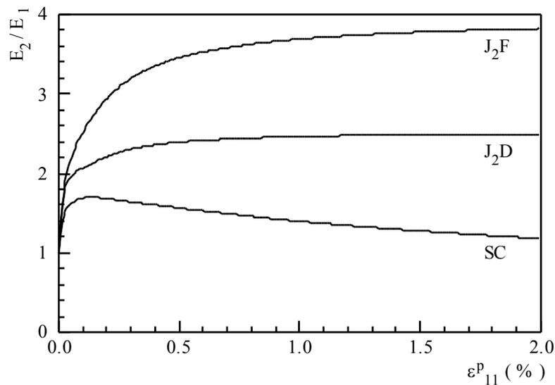
**Figure 4:** Evolution of the ratio  $E_2/E_1$  for the two phenomenological models  $J_2F$  and  $J_2D$  and for the self-consistent model SC.
