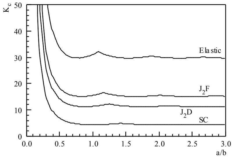
**Figure 8-a:**  $K_c$  versus aspect ratio  $a/b$  in the elastic case, for the two phenomenological models and for the self-consistent model when the applied plastic strain is 0.2%.
