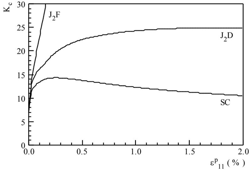
**Figure 7:**  $K_c$  versus plastic strain for  $a/b = 0.5$  for the two phenomenological models  $J_2F$  and  $J_2D$  and for the self-consistent model SC.
