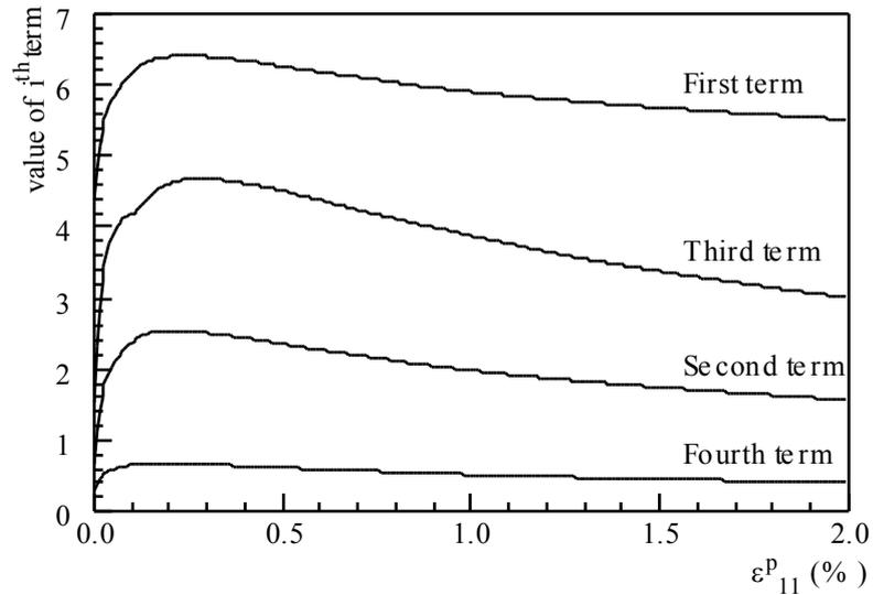
**Figure 10-a:** The four terms of  $K_c$  versus plastic strain according to self-consistent model SC and with an aspect ratio  $a/b = 0.5$ .
