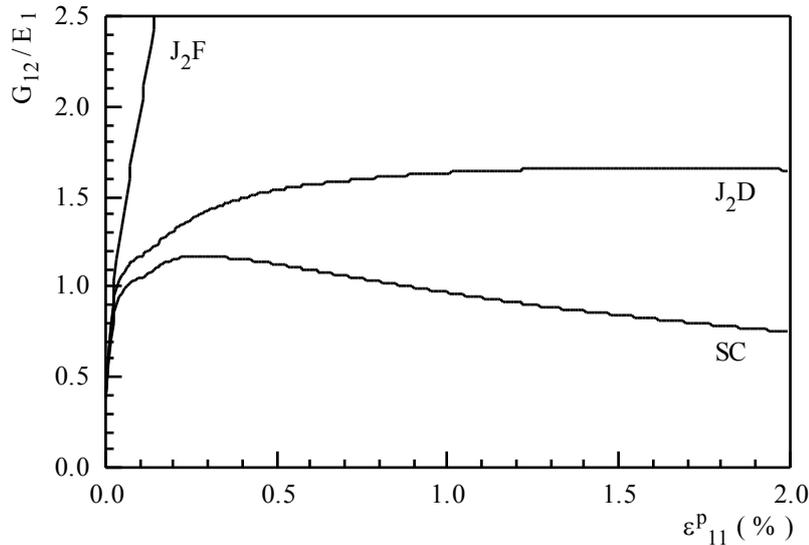
**Figure 5:** Evolution of the ratio  $G_{12}/E_1$  for the two phenomenological models  $J_2F$  and  $J_2D$  and for the self-consistent model SC.
