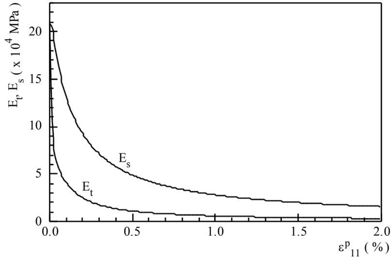
**Figure 3:** Evolution of the tangent and secant modulus deduced from the self-consistent model.
