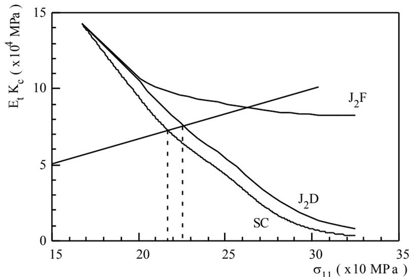
Figure 9:  $E_t K_c$  versus stress  $\sigma_{11}$  with an aspect ratio  $\frac{a}{b} = 0.5$ .
