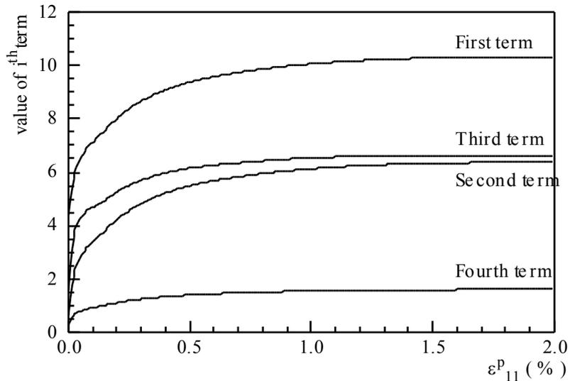
**Figure 10-b:** The four terms of  $K_c$  versus plastic strain according to  $J_2D$  theory and with an aspect ratio  $\frac{a}{b} = 0.5$
