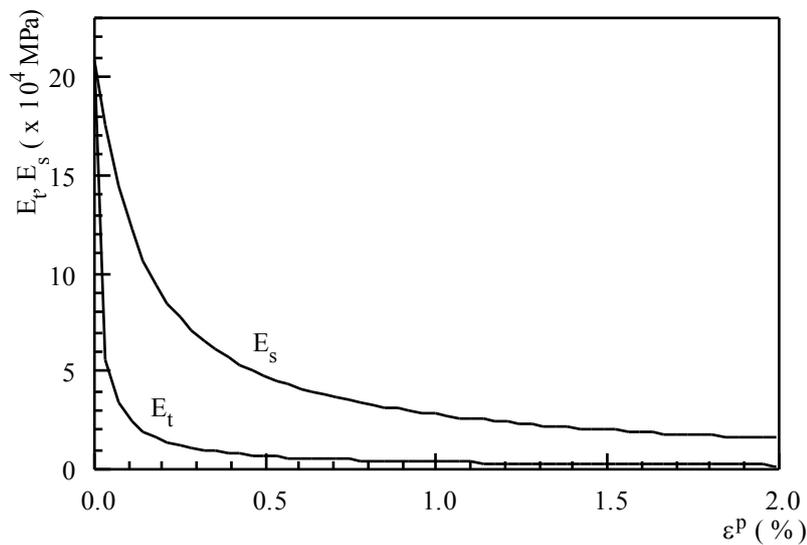
**Figure 1-2:** Evolution of the tangent and the secant modulus for the power law (8).
