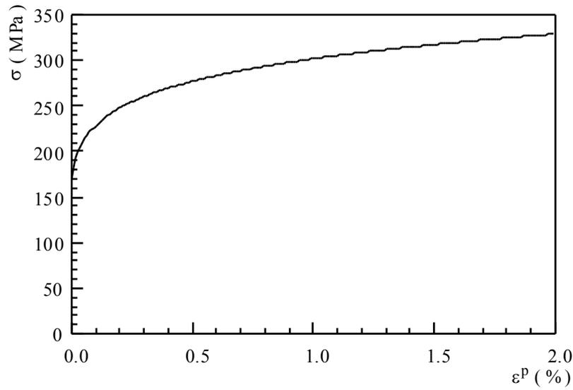
**Figure 1-1:** Stress strain curve for the power law (8).
