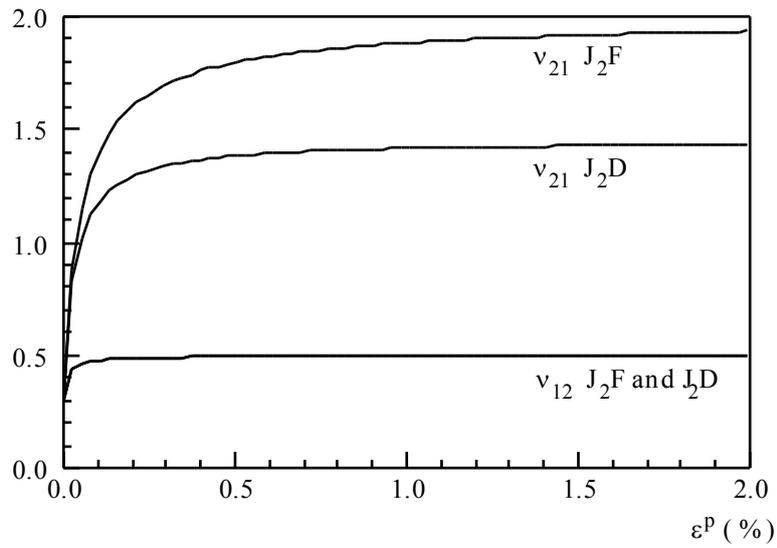
Figure 1-3: Evolution of Poisson ratios for the models J<sub>2</sub>F et J<sub>2</sub>D.
