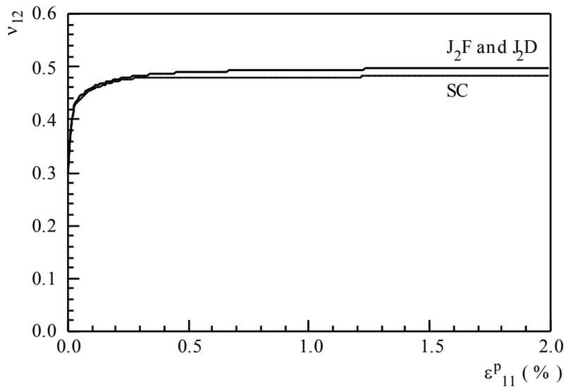
**Figure 6:** Evolution of the Poisson's ratio for the two phenomenological models  $J_2F$  and  $J_2D$  and for the self-consistent model SC.
